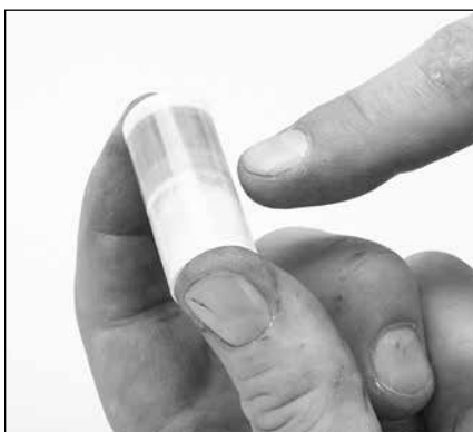
1.21 Inspect ceramic plunger for cracks and scoring to the surface. Clean with a wire-wheel brush if necessary.
