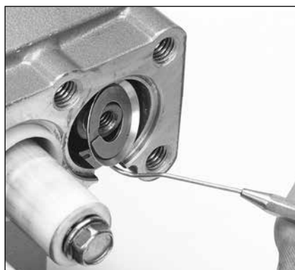
1.22 Use a pick to remove keyhole washer and barrier slinger located behind the plunger. Inspect for damage.
