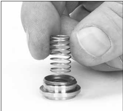
2.14 Place spring onto concave side of valve.
