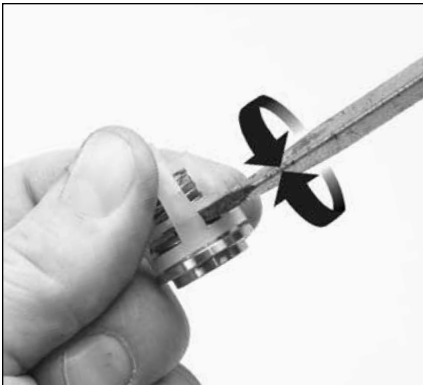
2.05 Insert flat tip screwdriver through spring retainer just above valve. Twist to create a small gap between spring retainer and valve seat.
