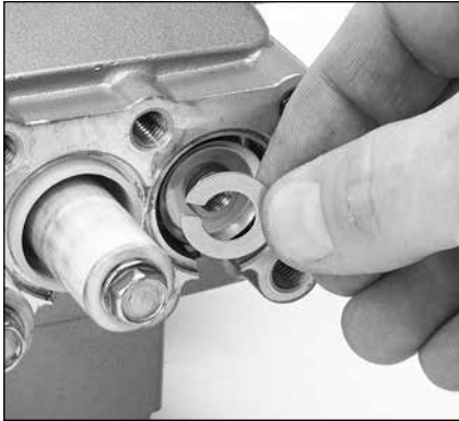
1.24 Install keyhole washer. The slot can face any direction.
