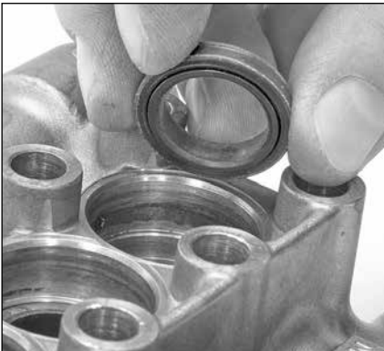
1.13 One side of the high-pressure seal has a groove. Install groove side facing down and press into place.
