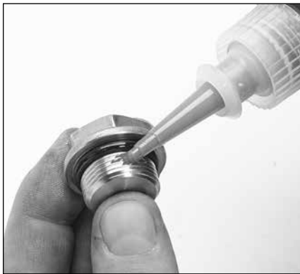
2.21 Place a drop of Loctite® 242® on the threads of valve plug.
