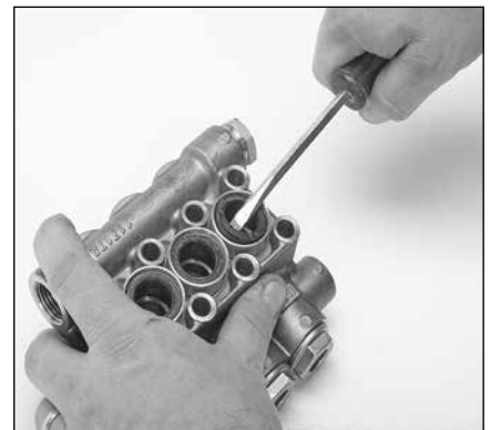
1.06 Use a flat tip screwdriver to pry the low-pressure seal upward and remove.
