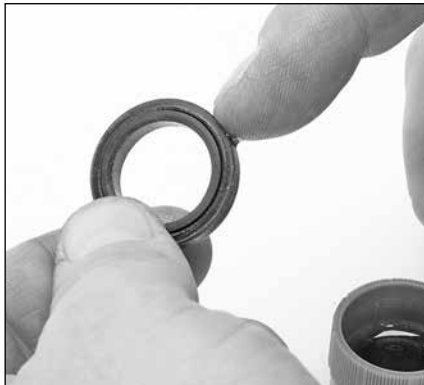
1.12 Apply a lubricant to the outside surface of the high-pressure seals.
