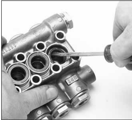
1.10 Use a flat tip screwdriver to pry the high-pressure seal upward and remove.
