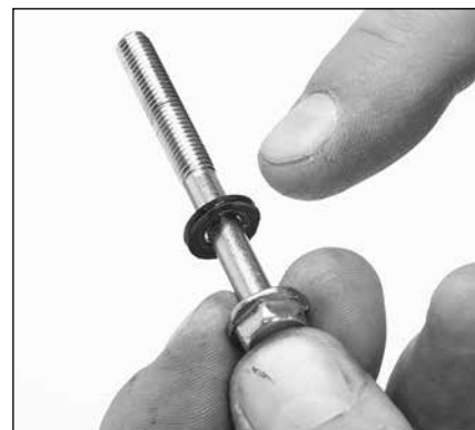
1.20 Remove and inspect plunger retainer gasket.
