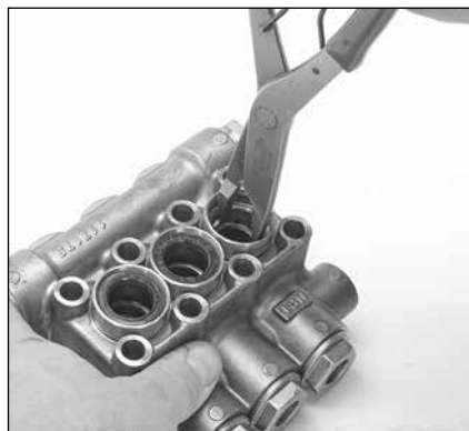
1.08 Using a reverse pliers, grasp second step of seal case. Remove with a twisting motion.
