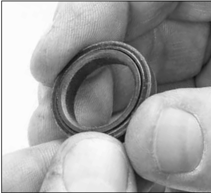
1.11 Inspect the inside diameter of the high-pressure seals for wear or damage.
