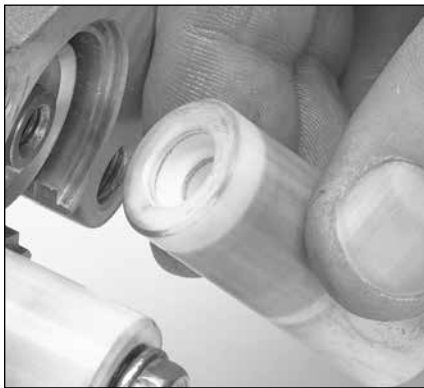
1.26 Look for stepped side of plunger. This side goes towards the pump crankcase.
