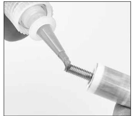
1.28 Place a drop of Loctite® 242® on the threaded end of the plunger rod.
