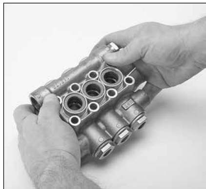
1.05 Place the manifold on a flat surface with low-pressure seals facing up.
