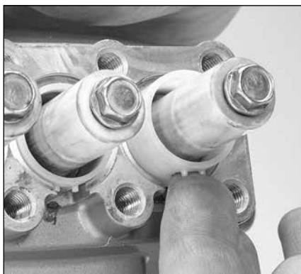
1.18 Remove seal retainers from crankcase housing.
