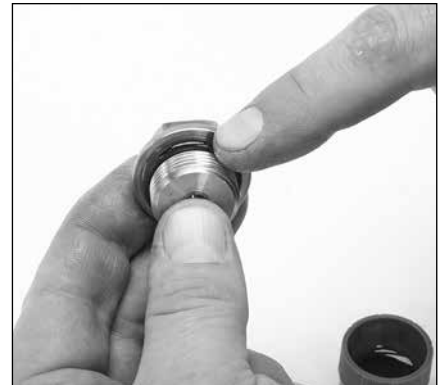
2.20 Replace valve plug O-ring with new one from valve kit and apply a lubricant to outside surface.
