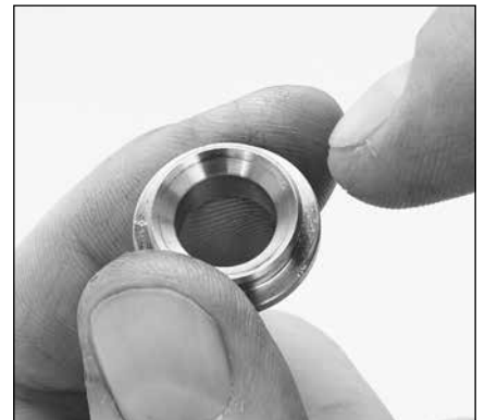
2.10 Inspect tapered surface of valve seat for wear, pitting or damage.
