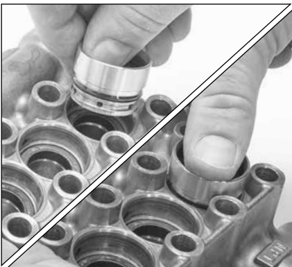
1.16 Install seal case with O-ring side down into the manifold. Press into place.
