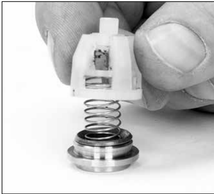
2.15 Place spring retainer onto valve seat.
