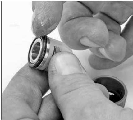
2.17 Replace valve seat O-ring and apply a lubricant to outside surface.
